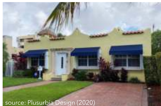
Current photograph of the Spanish Cottage at 2469 SW 22nd Terrace, featuring shaped parapets, elaborated chimney top, Spanish tile, rough stucco exterior, and a bell tower.
