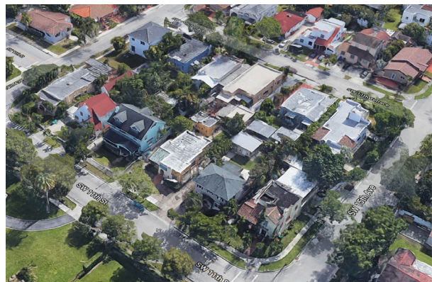
Figure 3.20: This aerial view of the 1400 block of 11th Street shows that nearly every house on the block has an ancillary building in the back. The block features the density of a multifamily neighborhood, with the appearance from the street of a suburban single-family neighborhood..
