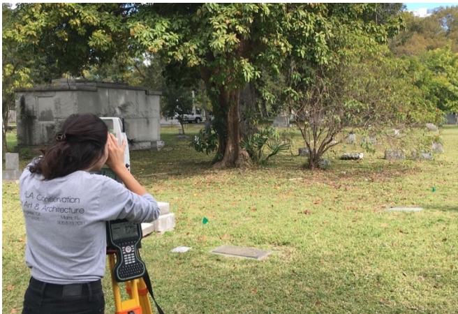
Using the Leica Total Station and other equipment to collect accurate point locations for each grave marker/monument. This produced a data set with GPS coordinates of each marker that was included on every survey form.
